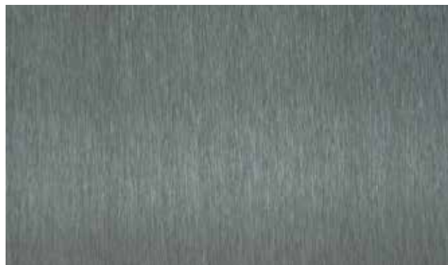
Satin finish - 180 grain vertical surface finishing Superficie satinata grana 180 verticale
