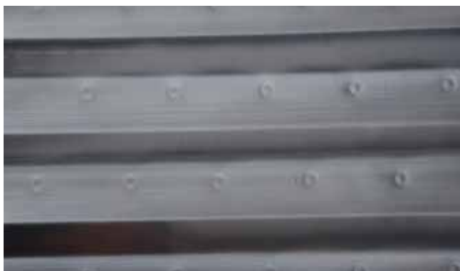
Termostar polished interior double wall, with repeated polishing of the sheet metal in the area of the studded seam.
