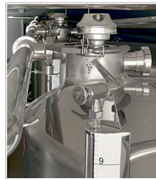
Chiusini con sfiato aria Stainless steel upper manways with vent valve
