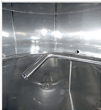
Decantatore interno Inside view of stainless steel racking decanting arm
