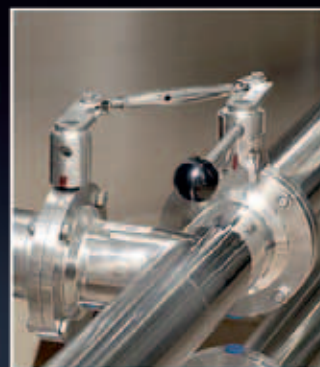
Valvole a farfalla tre vie Stainless steel 3 way butterfly valves
