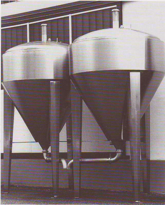
Maturatori termostatici a scarico agevolato Easy unloading temperature-controlled curers Thermostatische Reifungsbehältnisse
