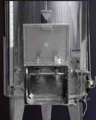
50 hl Criotank with insulated double door
